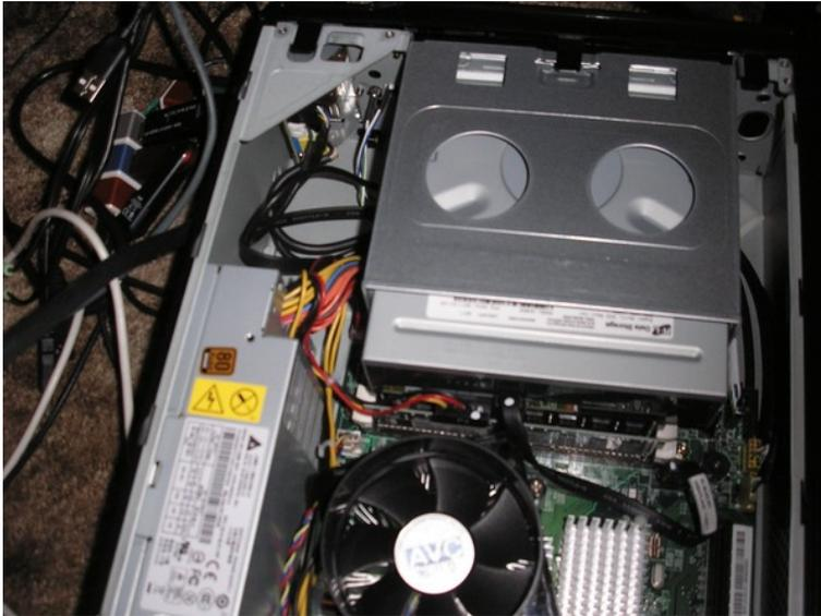
Gone are the wide ribbon cables. The cables for the SATA hard drive and DVD drive are smaller around than a typical power cord. The system also has a dual core processor, which greatly speeds up operations. Windows 7 has borrowed many items from Linux. It actually insists that you set up a password. Actually, the trial of the first system, before I returned it, was quite embarrassing! I actually forgot the password and was unable to get into my earlier eMachine.
