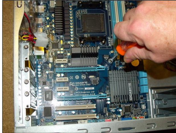
*Securing the motherboard in the new case.*
