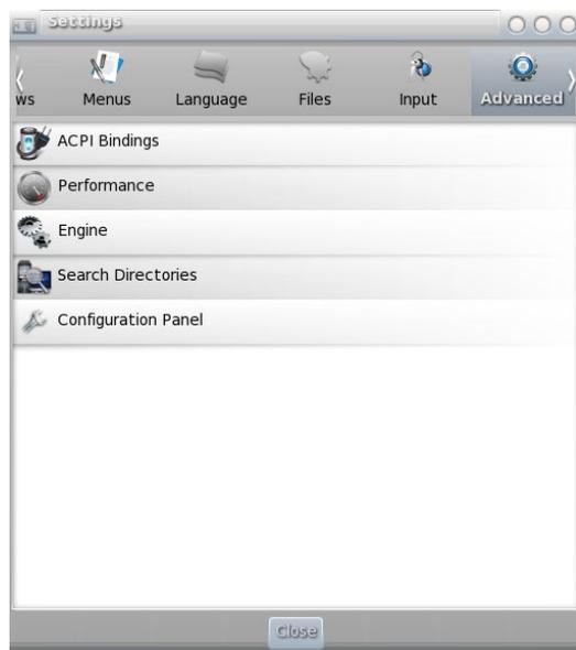
**ACPI Bindings** - This is a configuration you can use to tell the system what to do for certain keystrokes. For example, you can designate that the computer be suspended or shut down immediately if the power button is pressed. You can also choose what you want to do if your laptop lid is closed (shut down or hibernate or suspend). There are several defaults already in place.
