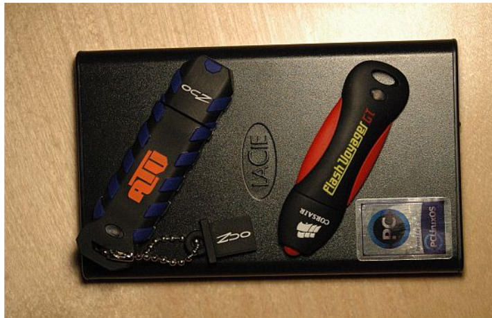
Figure 1: The testbed of external USB devices: 2 sturdy flash drives with fast write performance: OCZ ATV (32GB) and Corsair Flash Voyager GT (16GB) and the external slim LaCie Mobile Hard Drive II (250GB, 2.5").
